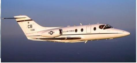
Beechcraft T-1A Jayhawk Max Speed – 330 kts Cruise airspeed – 250 kts; Pattern airspeed – 180 kts Final airspeed – 120 kts
